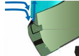
Internal chin pad with holes to adjust the airflow
