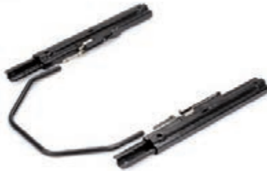
F3 Sliding tracks, travel 230 mm. No FIA. Z200002_A
